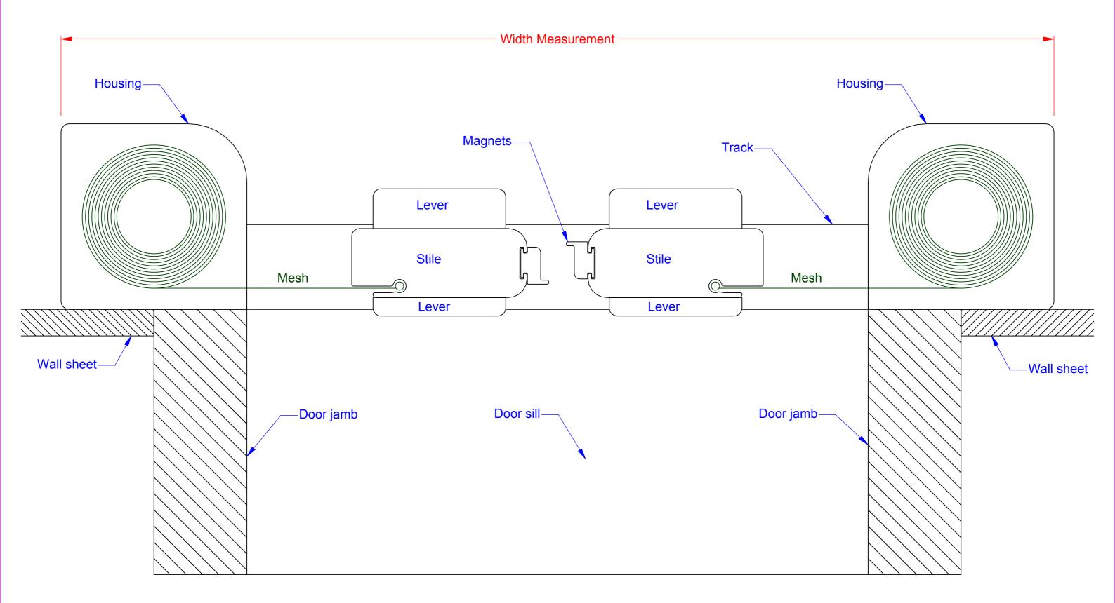
Freedom Screens Zipline PLAN VIEW - INTERNAL CORNER SCALE 1:2 at A3 Revision-007 Mesh Door sill-Width Dimension
